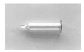
The heart of the PID or sensor is a lamp that emits photons in the vacuum-ultraviolet region. The lamp consists of an enclosure glass tubing, a crystal window which attached on glass tubing and filled gases in the enclosure tubing. The photon energy depends on the type of gas used to fill the lamp, and the crystal used as a transmission window.
