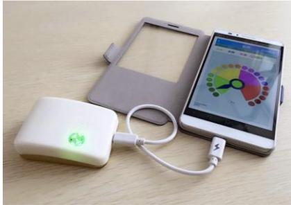
and  $\gamma$  detectors, SemeaAlert -Gamma is not built with a digital display. Instead it has a large LED and buzzer that change the color and number of beeps to indicate Normal, Low-Alarm, Mid-Alarm and High-Alarm representing radiation levels. This design not only helps the users who lack knowledge of radiation easily understand how strong the radiation is, but also tremendously lowers the product cost so that it becomes an affordable personal radiological protection device.
