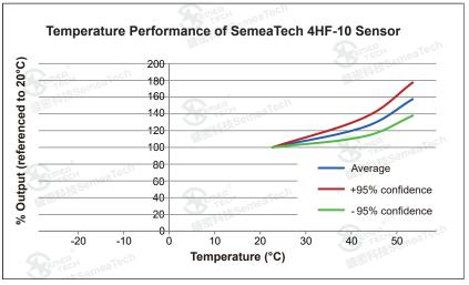
Note: Data for temperatures below 20 °C is unavailable due to the absence of a vapor phase for Hydrogen Fluoride at temperatures lower than this.
