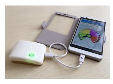
and  $\gamma$  detectors, SemeaAlert -Gamma is not built with a digital display. Instead it has a large LED and buzzer that change the color and number of beeps to indicate Normal, Low-Alarm, Mid-Alarm and High-Alarm representing radiation levels. This design not only helps the users who lack knowledge of radiation easily understand how strong the radiation is, but also tremendously lowers the product cost so that it becomes an affordable personal radiological protection device.
